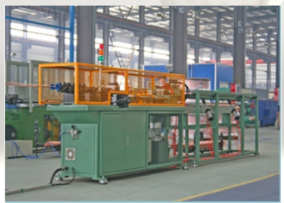
Straightening and cutting machine
